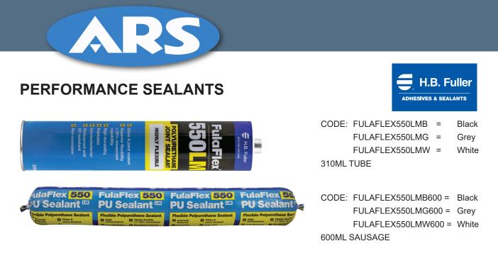
**FulaFlex**<sup>™</sup> **550LM** is a one component moisture-curing low modulus Class A polyurethane sealant with excellent joint movement capabilities. It cures to form a flexible, durable and weather proof sealant and exhibits excellent adhesion to a wide range of common construction substrates. FulaFlex<sup>™</sup> 550LM is paintable and satisfies the requirements for the Green Building Council of Australia (GBCA).
